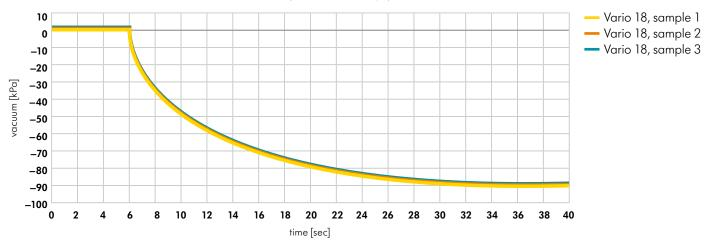
Vacuum build-up, Vario 18 AC, calculated at sea level (with filter and 1 L jar)
