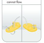
5 Screw the assembled tube and clamp onto the TwistLok lid.
